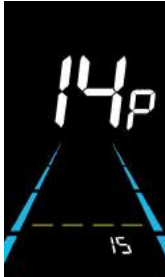
Figure 6-14 Controller current limit setting interface
