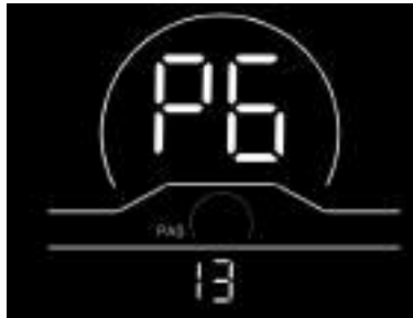
Fig. 4-6 Current Limit Setting Interface
