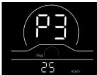
Fig. 7-3 Speed Limit Setting Interface
