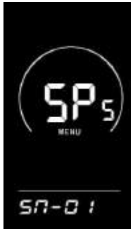
Fig. 8-9 Steel Magnet Selection Interface for Speed Sensor
