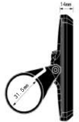
Fig. 3-4 Side View of Display 80C Dimensions
