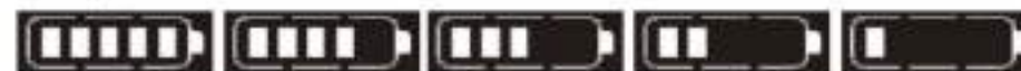
Full battery level indicator 4-segment indication 3-segment indication 2-segment indication 1-segment indication
