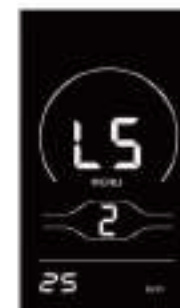
Fig. 7-2 Speed Limit Setting Interface
