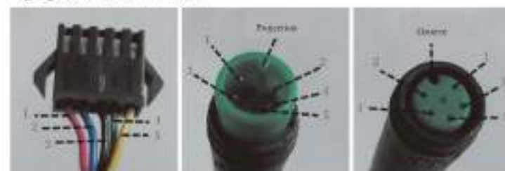
Connecting terminal to the controller
